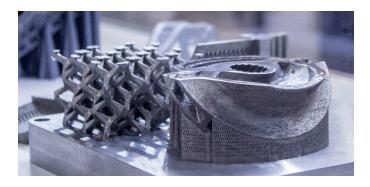
Manufacturers from aerospace and automotive, to medical devices, are now 3D printing production metal parts using a variety of processes. However, metal printed parts typically require post-processing operations in a furnace to bring components to their final dimensions and properties. Multiple variables must be considered when choosing a furnace, including the print technology, part design, size, material, and the volume of parts to be produced.
