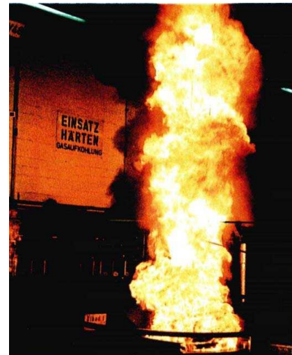
Figure: High flames during oil quenching in case of pit furnace installation
