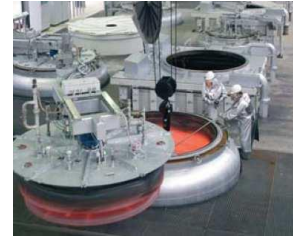
Pit Furnace Installation
